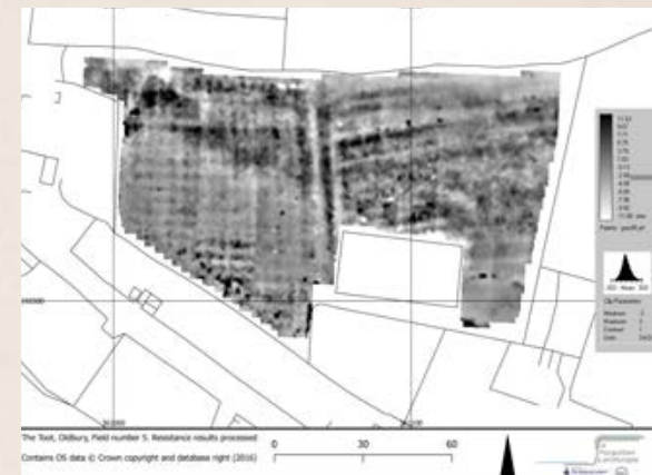
Geophysical results from one of the fields, the shading reflects the pattern of the earth resistance. The vertical light and dark bands in the middle show an old field boundary. The light results on the bottom left represent the "palaeochannel" of the Severn (© AFL 2017)
